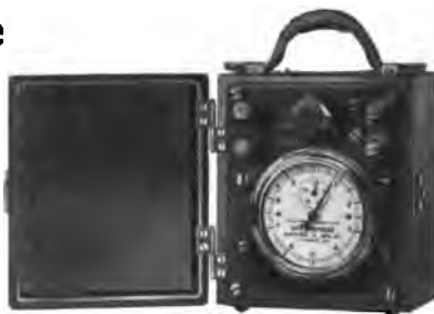
Westinghouse Portable Standard or checking single and polyphase watt-hour meters
